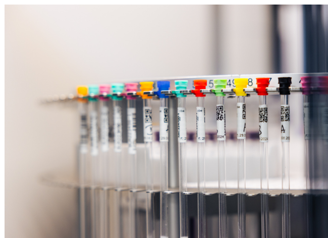
Fig.2: Automated sample jet holder of the NMR spectrometer, enabling high-throughput analysis
